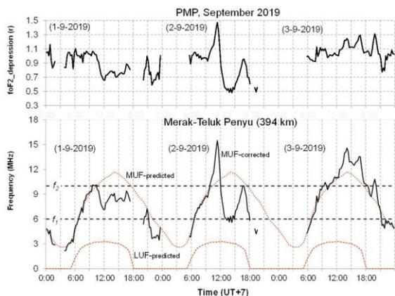
Fig.7. The graph of  $foF2$  depression ( $r$ ) above Pameungpeuk from September 1 to 3, 2019 (top panel) and the correction results for MUF predicted using ASAPS software, for the Merak - Teluk Penyu communication circuit.
