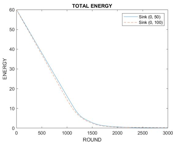
Fig.11. Total Energy of 100 Nodes with Sink Position (0, 50) and (0, 100)
