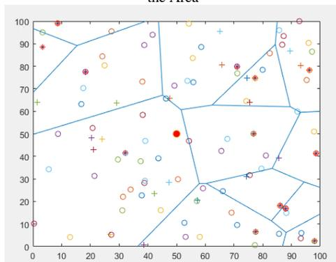
Fig.2. Distribution of 100 Nodes at the Sink Position in the Center Area
