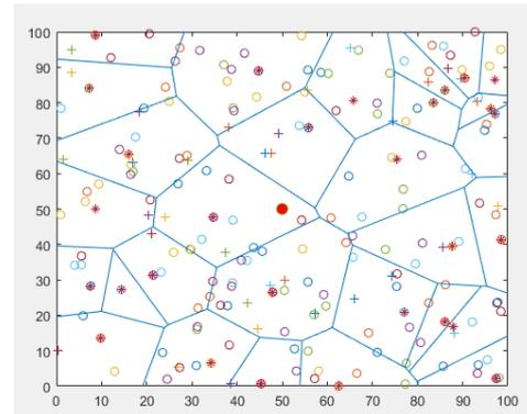
Fig.4. Distribution of 200 Nodes at the Sink Position in the Center Area
