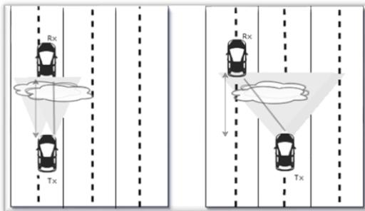
Fig.5. The process of communication with interference from the fog weather.
