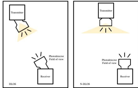
Fig.1. Illustration of communication channel model line of sight.
