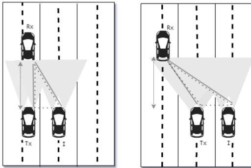
Fig.4. The process of communication between vehicles plus light interference from one vehicle.
