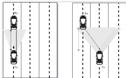
Fig.3. Communication between vehicles without light interference.
