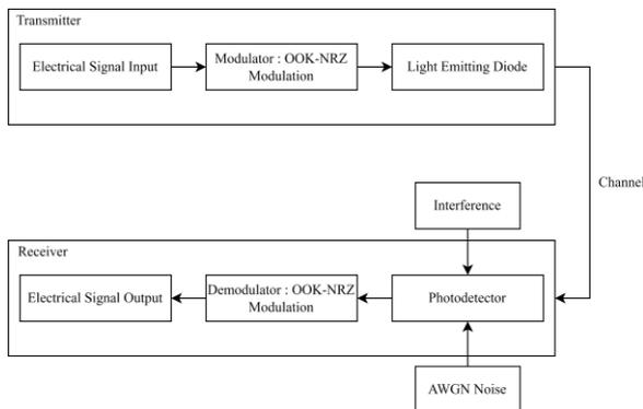
Fig.7. Diagram of communication systems between vehicles.
