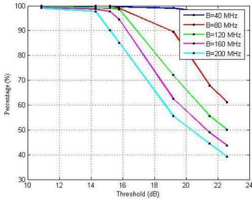
Fig.7. The Coverage Percentage When Transmitter Power 0.01 Watt
