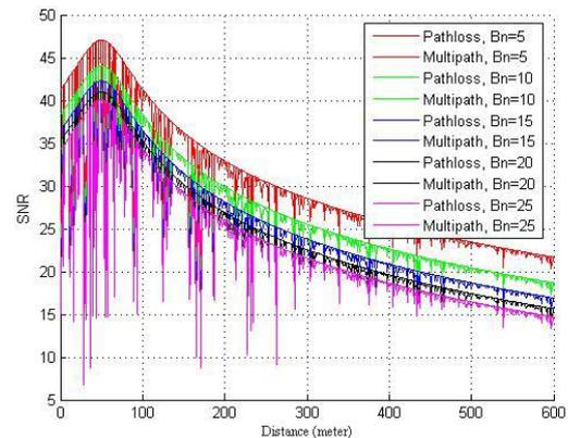
Fig. 4. SNR for Transmitter Power 0.01 Watt
