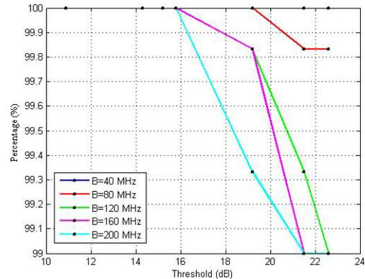
Fig.8. The Coverage Percentage When Transmitter Power 0.1 Watt
